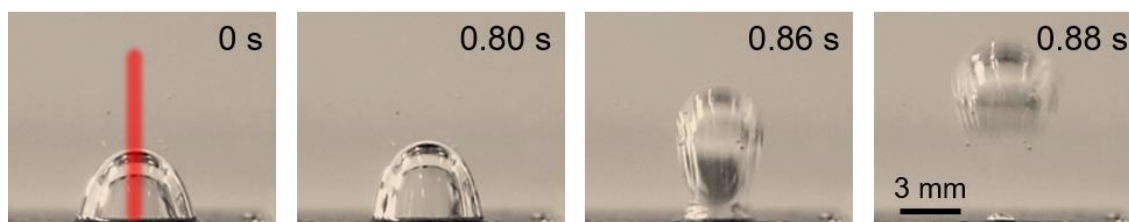
Supplementary Figure 14 | Sequential images showing the bubble detachment from the PESS under NIR irradiation.
