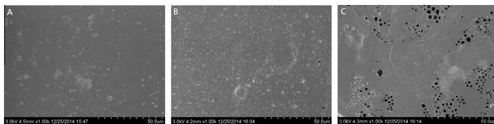
Figure 6 SEM photographs showing surface morphologies of RI. (A) Before drug release; (B) after 3-day drug release; (C) after 12-day drug release. All photographs were obtained at 1000 \times magnification.
