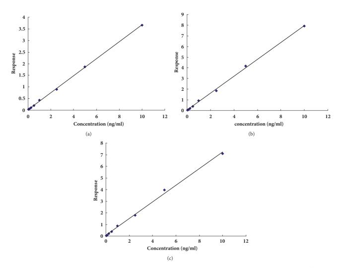
FIGURE 5: Standard curves of aconitine, mesaconitine, and hypaconitine in biological samples. (a) aconitine, Y = 0.3651X + 0.021,  $R^2 = 0.9997$ ; (b) mesaconitine, Y = 0.7952X + 0.0218,  $R^2 = 0.9987$ ; (c) hypaconitine, Y = 0.718X + 0.0605,  $R^2 = 0.9970$ .
