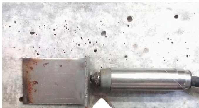
Figure 3. LVDT positioned at the side face of a specimen to measure the crack size at the height of the embedded capsule.
