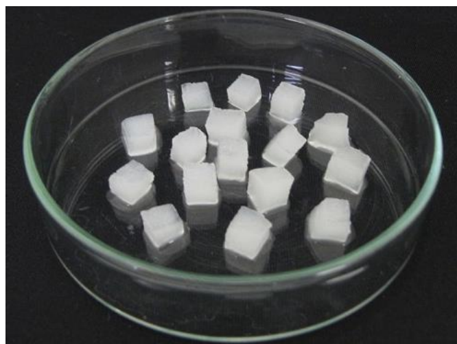
Figure 3. Immobilized enzyme prepared with \kappa -carrageenan. Immobilized enzymes were prepared using 1.5–4.0% ( w/v ) \kappa -carrageenan and crude enzymes AlyFRA or AlyFRB, which were cut into cubes of approximately 5 mm.
