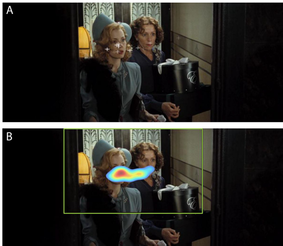
Fig. 2. Example of democratic COI determination. (A) Gaze locations of the 24 participants during one frame of one video clip. (B) Kernel density estimate of those gaze locations in that video frame shown as a heat map, with red representing a higher density. The green rectangle represents the box used to determine the democratic COI.
