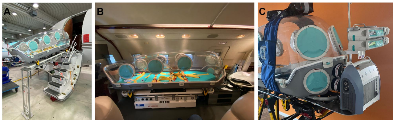
Figure 1 EpiShuttle PMIU in a Bombardier Challenger 604 Air Ambulance Jet. Panel (A) Loading/Unloading of the EpiShuttle PMIU. Panel (B) The EpiShuttle PMIU in the Cabin of the Challenger 604. Panel (C) Equipment "Rack" at the Head End of the EpiShuttle PMIU and "Saddle" to prevent disconnection of lines, ventilation tubes and monitoring during loading and unloading.
