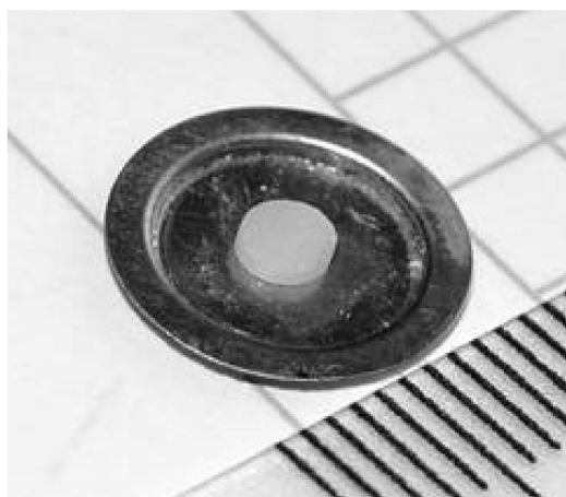
Figure 1. An exemplary \text{LiMgPO}_4 (LMP) crystal grown from melt using the micro-pulling-down method. The crystal was placed on a stainless steel cup that held the sample during luminescence measurements inside the Risø TL/OSL DA-20 reader.
