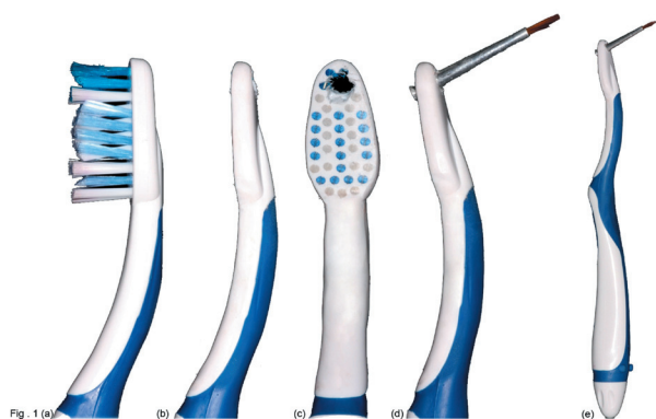
Figure 1- Step-by-step fabrication of the portable device designed to casting plaster (a): electric toothbrush; (b): bristles of the brush removed; (c): hole on tip of the toothbrush in place of the bristles; (d): installation of the tip of a brush on the opposite side of the bristles and (e): portable vibrator ready
