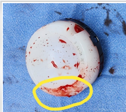
Figure 5: Damaged liner with yellow circle probably due to disengagement of glenosphere.
