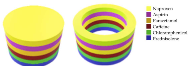
Figure 1. 3D designs of the printlets. Type I: Cylinder (left, 10 mm diameter and 3 mm height), Types II and III: Ring (right, 10 mm diameter and 6 mm height).
