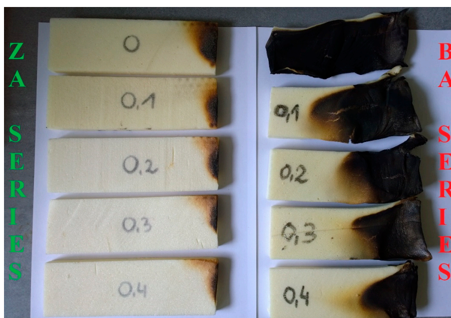
Figure 9. Appearance of ZA and BA series of foams after horizontal burning test.
