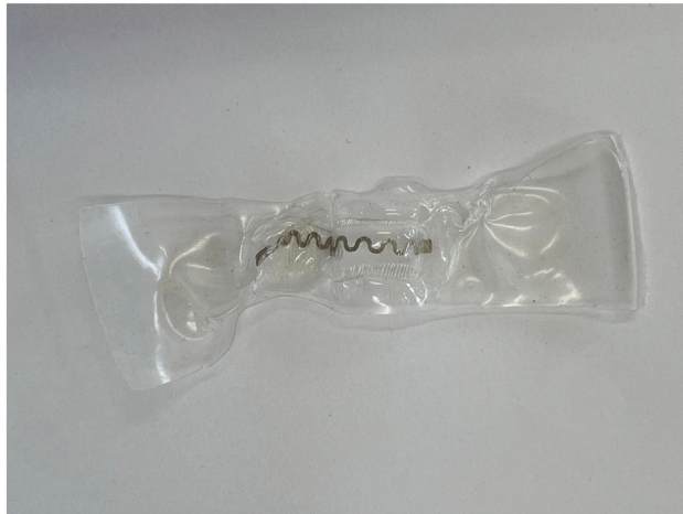
Figure 12. A deformed SIS substrate with the Ag NWs electrode after heating at 80°C
