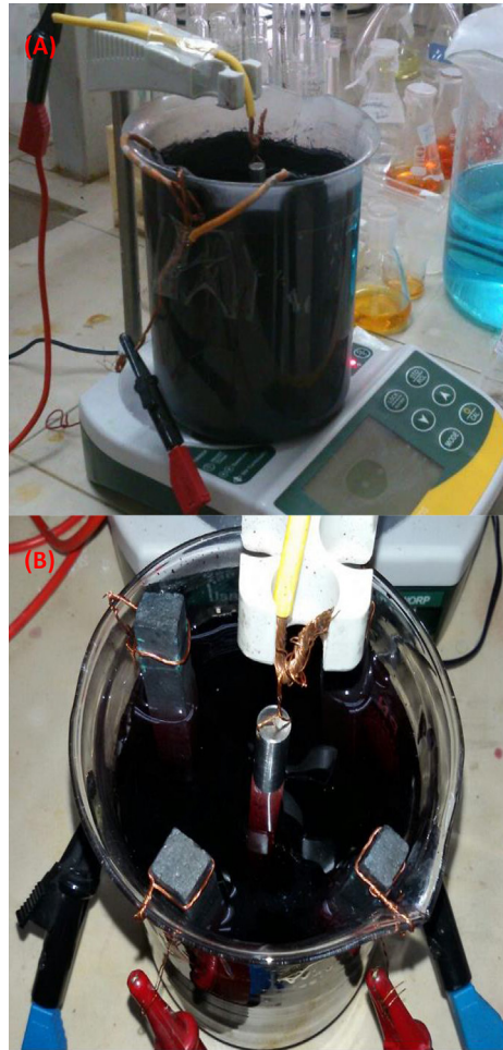
Fig. 20. Coating bath, (A): coating bath with anodic graphite paste, (B): coating bath with insoluble anodic graphite.
