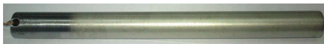
Fig. 25. Industrial iron electrodes, which has been coated with tin in the appropriate operating conditions.
