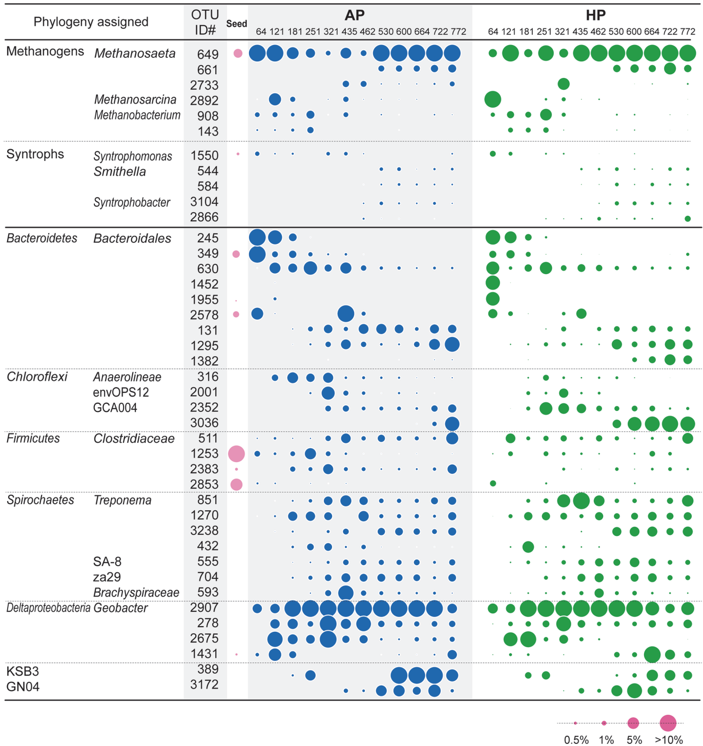
Fig 4. Bubble plot indicates the relative abundances of major OTUs retrieved from anaerobic packed-bed (AP) and hybrid packed-bed (HP) reactors. The numbers below AP and HP on top row indicate days of the operation for biomass sampling.
