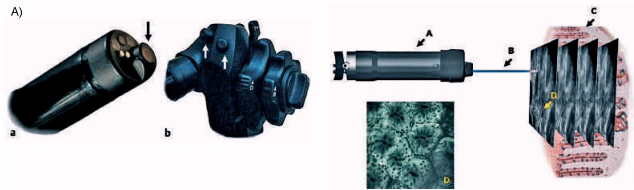
Design of a confocal endomicroscopy: a confocal laser microscope protrudes 2 mm out of the distal tip of the endoscope and is manipulated by two additional buttons (left). Blue laser light penetrates the tissue and is reflected. Focusing on different depths yields optical sections at different levels (right).
