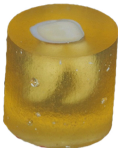
Figure 1. Prepared tooth embedded in epoxy resin after polishing with waterproof sandpaper and rinsing.
