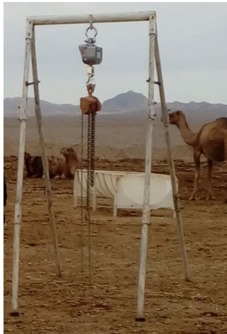
Figure 1. The portable weighting scale (Company: Fuzhou Kejie Intelligent Technology Co.,Ltd. model: OCS-XZ-2, 2000 Weigh Capacity (Kg), Accuracy Class III, +/- 1 division (least count). This were made from 13 pieces of iron, hanging digital scale 2000 kg, and one chain crane.
