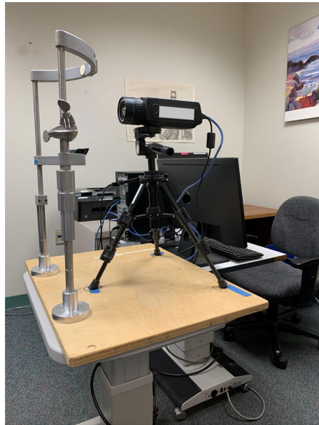
Figure 1. FLIR thermographic camera setup.
