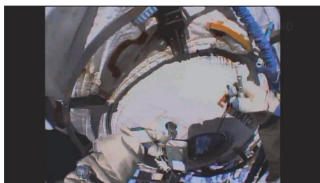
FIGURE 1: The process of sampling with sampler "TEST." Astronaut holds the body of sampler "TEST" in his left hand and the tampon holder screwed out in the open space in the right hand.
