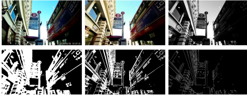
Figure 2. Digital image processing for the analysis of image characteristics. Top row: Left - original recording, middle - undistorted, white balanced, and de-noised image, and right - linearized greyscale image. Bottom row: Left - local entropy (texture), middle - high frequencies, and right - edges.
