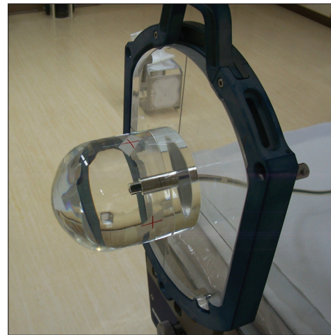
Figure 1: Dose validation acrylic test tool for verification of SRS treatments
