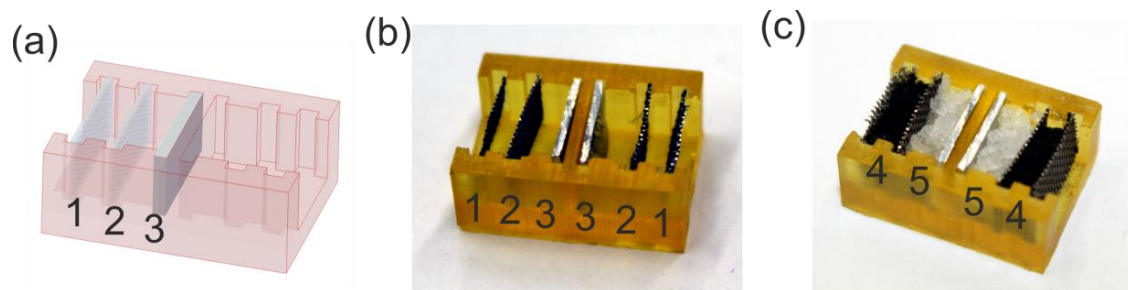
Figure 1. 3D-printed battery with distinct electrolyte chambers. (a) Battery design showing two individual battery parts with two platinum-coated meshes (1, 2) and one aluminum sheet (3). (b) Printed battery with platinum meshes (1, 2) and aluminum sheets (3). (c) Fully assembled battery from (b) with additional charcoal (4) and superabsorber/potassium hydroxide filling (5).
