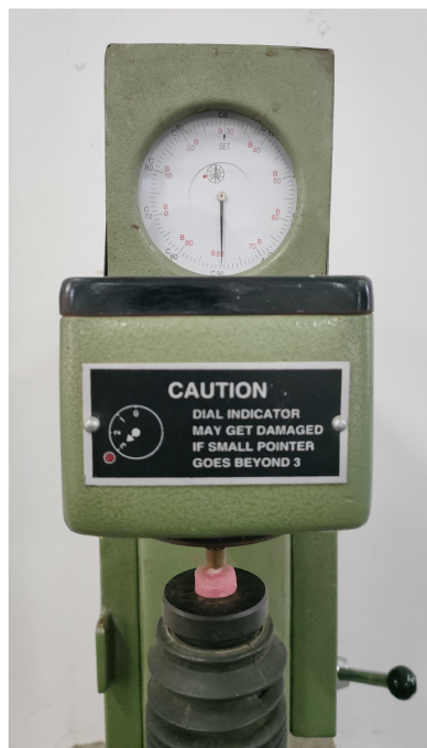
Figure 1 Brinell hardness testing machine with sample loaded.
