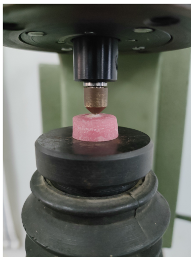
Figure 2 Microhardness indentation on the sample.
