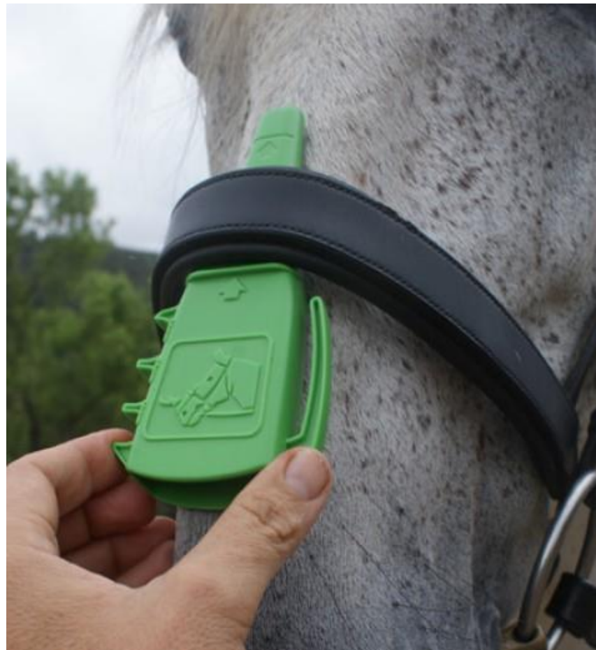
Figure 1. The ISES Noseband Taper Gauge being used to measure a noseband on the frontal nasal plane of the horse—the raised stop mark indicates how far the device should be able to be inserted under the noseband to indicate proper two-finger (1.5 cm) fit. Photo courtesy of ISES.
