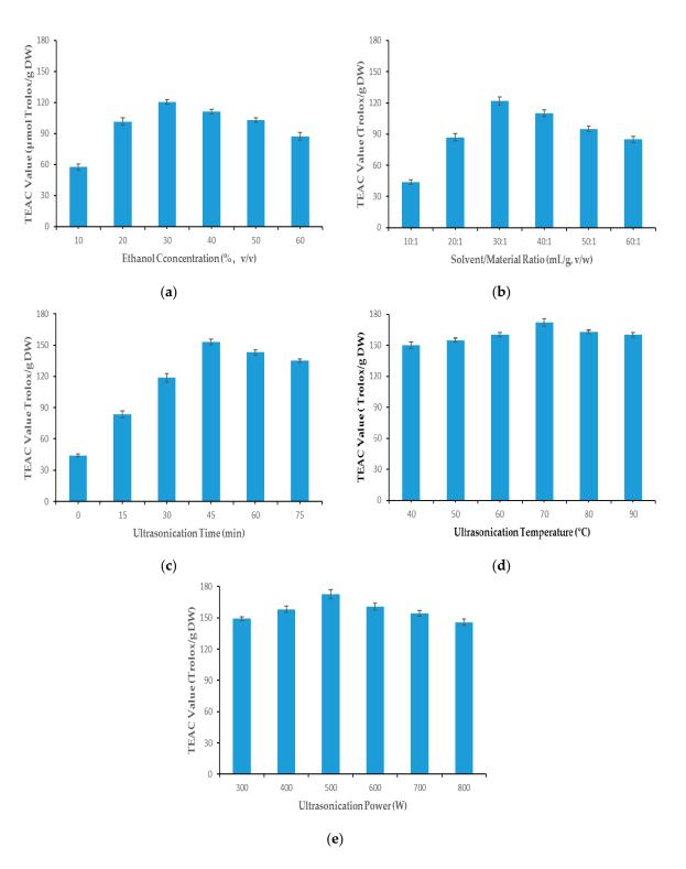
**Figure 1.** Single-factor experiments results: (**a**) Ethanol concentration; (**b**) Solvent/material ratio; (**c**) Ultrasonication extraction time; (**d**) Ultrasonication extraction temperature; and (**e**) Ultrasonication power.
