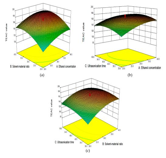
**Figure 2.** RSM analysis for UAE of antioxidant ingredients from GMBC in relation to concentration of ethanol and S/M ratio (**a**); concentration of ethanol and ultrasonication extracting time (**b**); S/M ratio and ultrasonication extracting time (**c**).
