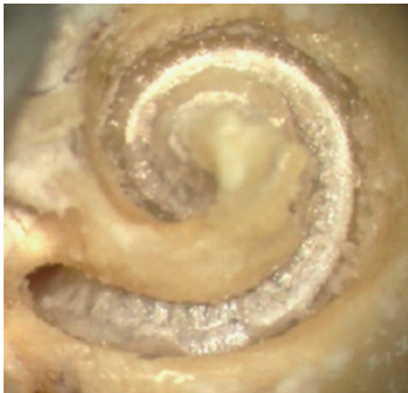
FIGURE 4: Cochlea with prepared basilar membrane before pull-out. CI array positioned under the BM.
