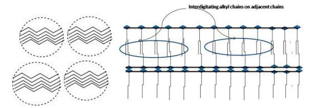
**Scheme 4.** Schematic of the crystalline alkyl chain domains (LHS) formed duetoaggregation behavior of alkyl chains on alternate repeat units (RHS of scheme).
