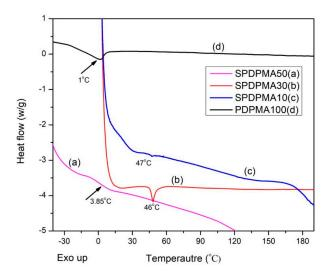
**Figure 5.** DSC curves of Styrene- PDPMA copolymers synthesized via one pot ATRP copolymerization (The  $T_g$  of poly (PDPMA) was = 1 °C [30] and poly (styrene) = 106 °C).
