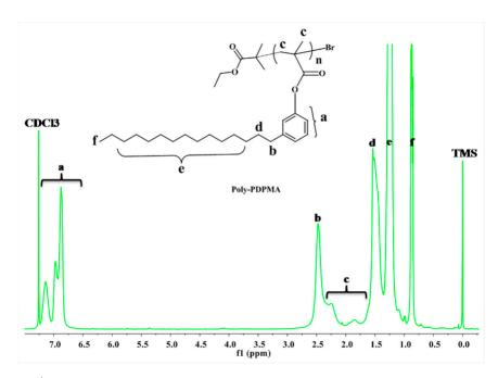
**Figure 1.** <sup>1</sup>H NMR spectrum of pentadecylphenylmethacrylatehomopolymer (poly PDPMA).
