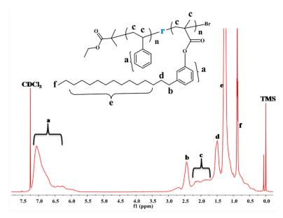
Figure 2. NMR spectrum of styrene-PDPMA copolymer (in the feed ratio 70:30) in CDCl<sub>3</sub>.
