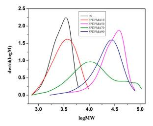
**Figure 4.** dwt/dlogM vs. log  $M_w$ plots of styrene-PDPMA copolymers showing variation in mol.wt. distribution as a function of the feed composition.
