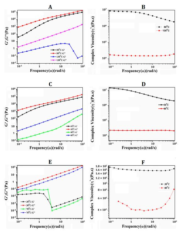
**Figure 8.** Variation in storage modulus (G'), loss modulus (G") and complex viscosity ( $\eta^*$ ) of styrene-PDPMA copolymers of varying styrene content at different temperatures. (Strain rate: 0.5%). Feed ratios for figures are, (**A,B**)—Styrene  $_{70}$ –PDPMA  $_{30}$ , (**C,D**)—Styrene  $_{50}$ –PDPMA  $_{50}$  and (**E,F**)—Styrene<sub>30</sub>–PDPMA  $_{70}$ .
