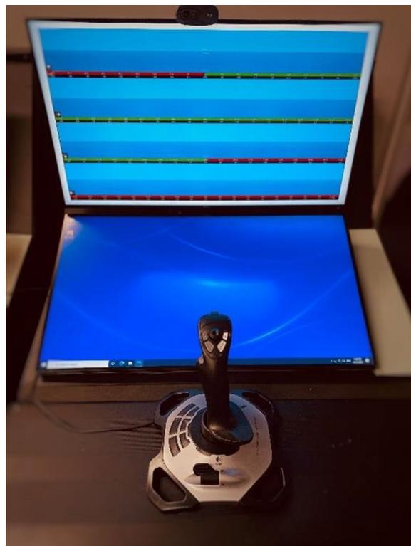
**Fig. 2** Panoramic display shown in top display, with response joystick in front. The bottom display was left blank during the tasks. The clockwise configuration is shown
