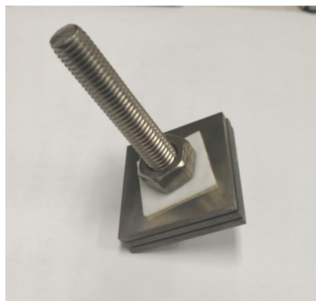
Figure 18. Crevice corrosion specimens of titanium alloys used in tests.
