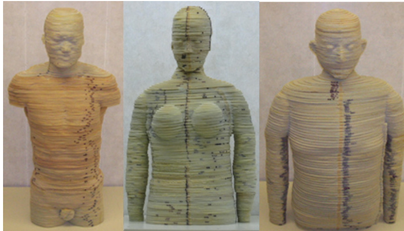
FIG. 3. (a) Phantom based on a segmented CT data set of an adult male; (b) phantom based on a computational adult female hybrid data set; (c) phantom based on a computational adult male hybrid data set.
