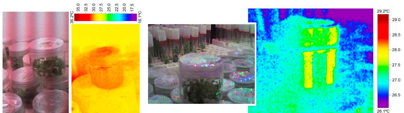
Figure 7. Thermographic images of the temperature in the vessels under (a) Gro-lux fluorescent lighting and (b) LED lighting. (Thermographic camera model 875. Manufacturer Testo).
