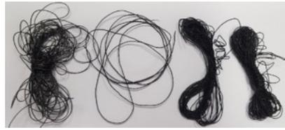
**Figure 1.** Coils of extruded composite fibers. From left to right, FGGr (Gr/SBS), FCNT (CNT/SBS), FM1 (CNT/Gr/SBS), FM2 (CNT/Gr/SBS) are shown, respectively.
