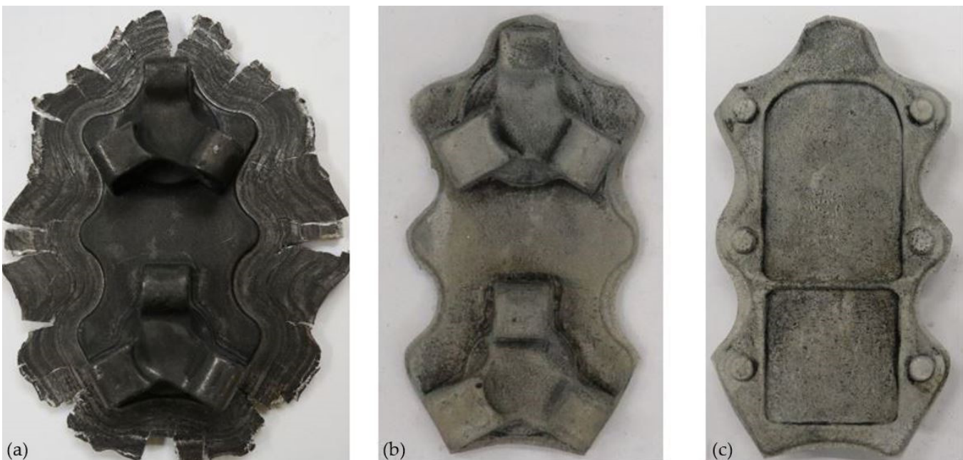
Figure 15. Forging obtained for a preform with a higher degree of forging (variant II): (a) after forging, (b) top view after trimming, (c) bottom view after trimming.
