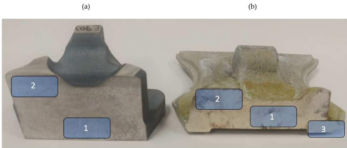
Figure 8. Microstructure test areas, (a) preform, (b) forging.
