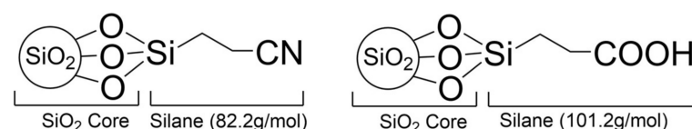
Figure 12. Schematic representation of the silica beads.
