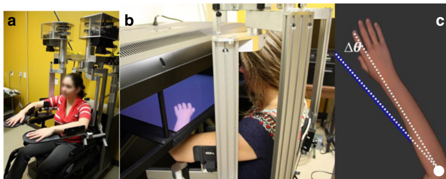
Fig. 1 KINARM Exoskeleton Lab. a Modified wheelchair with each arm supported against gravity by exoskeletons; b Virtual reality display; c Virtual arm and real arm positions (blue line; non-visible for the participant) where \Delta\theta represents the angular difference between the real and the virtual arm. The white circle corresponds to the center of rotation, i.e. the elbow joint
