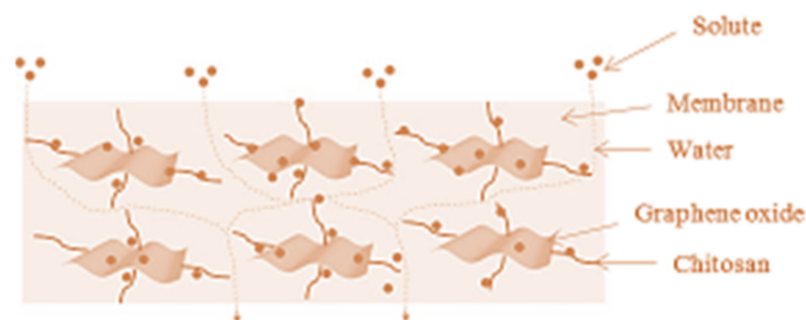
Figure 16. Graphene oxide–chitosan dispersion in water filtration membrane and its feed transport route. Reprinted from [42]. Copyright 2018 with permission from Elsevier.
