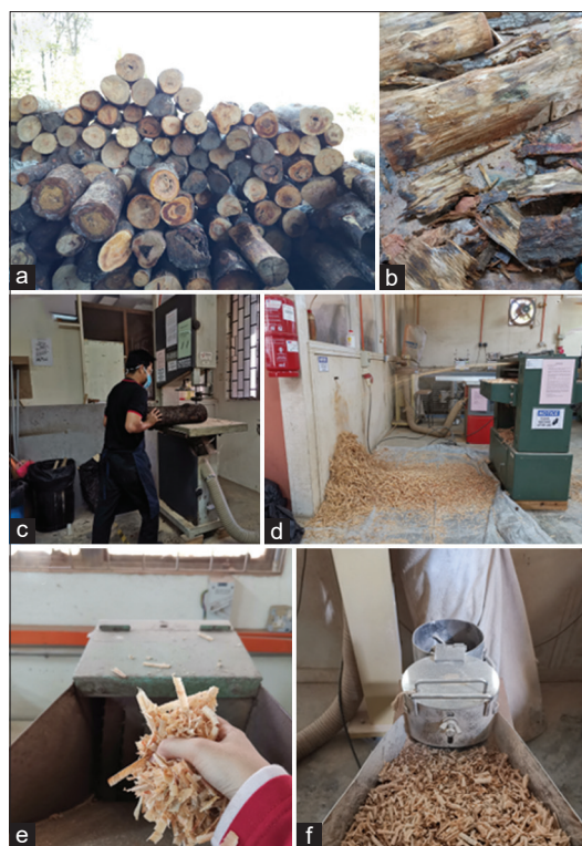
Figure 1: (a) Wood truck collected from mangrove factory, (b) Debarking process of the wood trunk, (c) Wood trunk was cut into two, (d) Planing process to produce wood particles, (e) Wood particle underwent grinding process, (f) Further grinding process to produce smaller wood particles ( \leq 500 \mu\text{m} )
