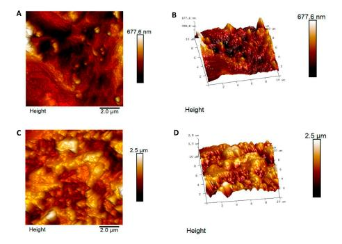
**Figure 1.** (A,C) Topographical and (B,D) Three-dimensional Atomic Force Miscroscopy (AFM) pictures of machined titanium surface (CTRL, upper line) and dual acid etched titanium surface (TEST, bottom line).
