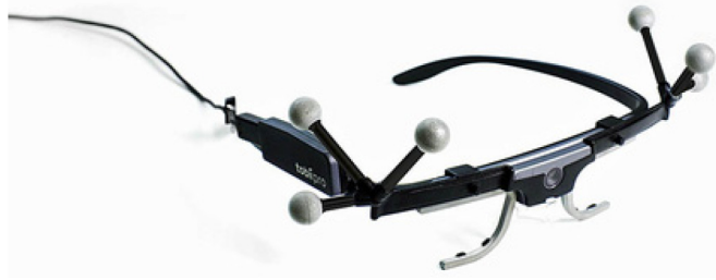
Figure 2. Tobii Pro glasses 2 with motion capture markers attached (Tobii, 2018).
