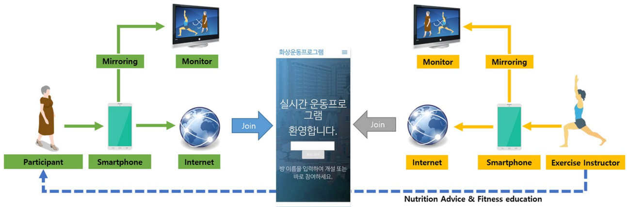
Fig. 2 Overview of the telepresence exercise platform using web real-time communication technology developed for this study in obese older women
