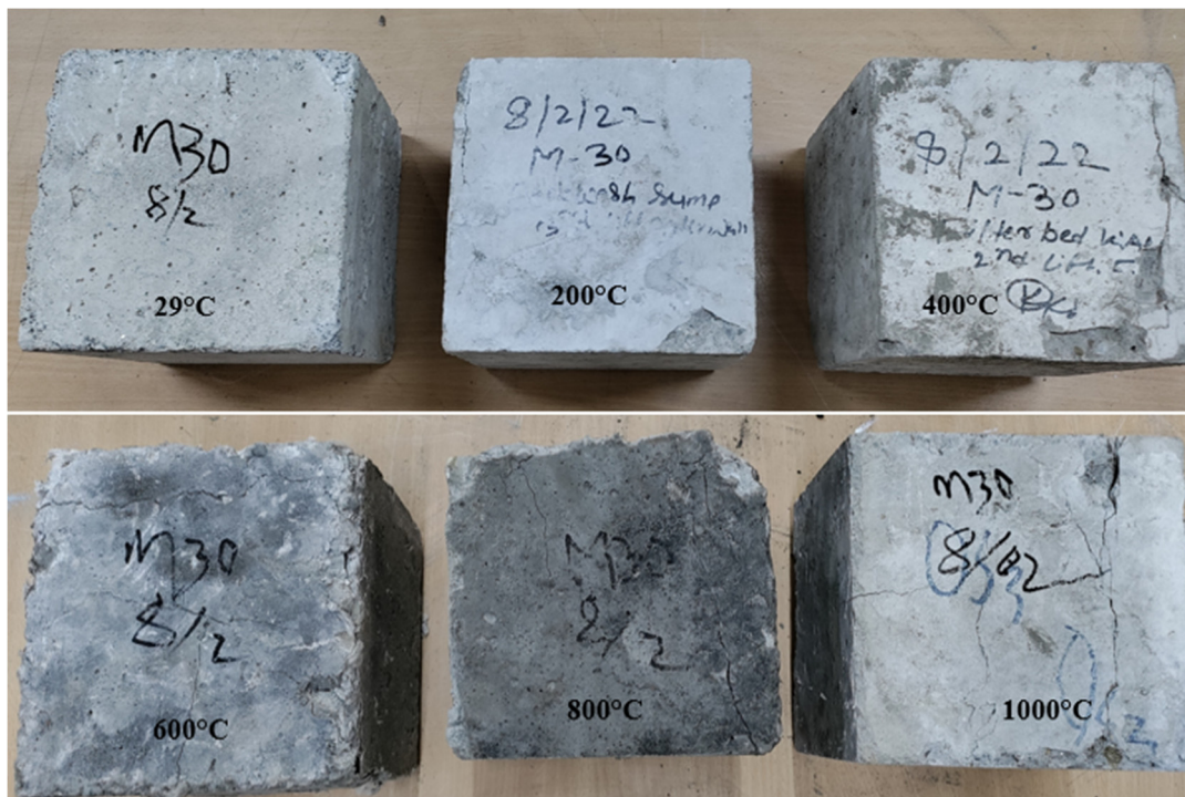
Figure 4. Concrete samples after elevated temperature.
