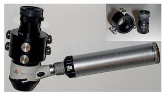
Fig. 1. Zeiss monocular used as a magnification tripler fitted through custom adaptor ring onto the Heine Delta-20; Inset: Zeiss monocular 3x12T\* and custom adaptor ring.
