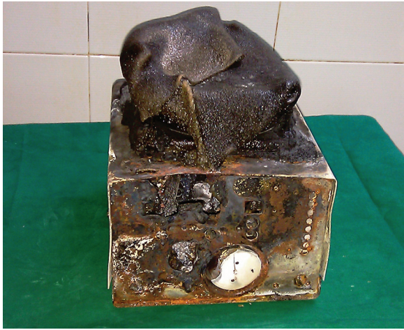
Figure 1: The melted and charred parts of the excel anaesthesia ventilator
