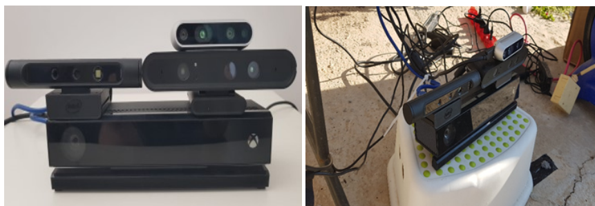
Figure 1. The setup of the four sensors used in the experiment. Kinect II at the bottom, the Astra Pro on the left, the SR300 on the right, and the gray D435 on top of the SR300.
