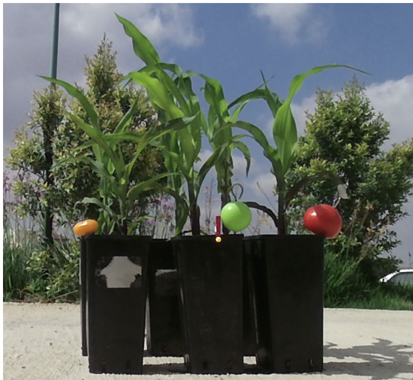
Figure 2. The experimental setup as captured by the Kinect sensor from 1 m. Six corn plants in black plastic pots arranged in two rows. Added tomatoes—a red tomato, an orange cherry tomato. Two plastic balls for size measurements—a larger green ball and a smaller yellow ball.
