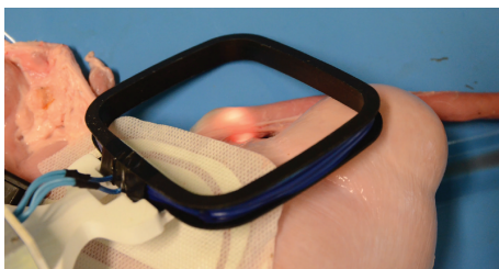
FIGURE 5: Powering the implant using wireless inductive power transfer.
