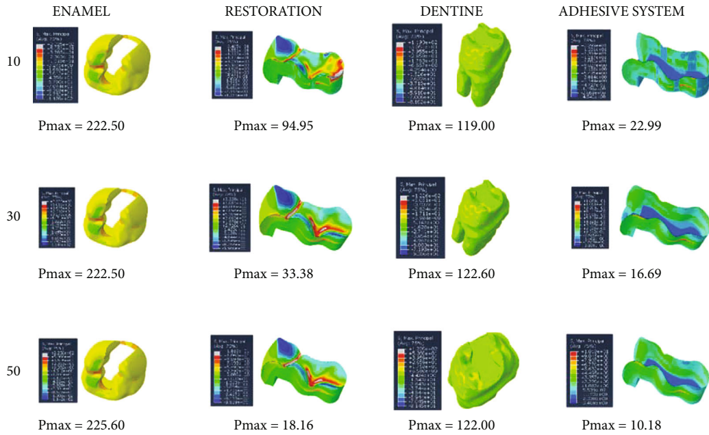
FIGURE 13: Stress distribution regions in a tooth with a class II disto-occlusal cavity when using adhesive system 4 with a thickness of 10, 30, and 50 micrometers, respectively.
