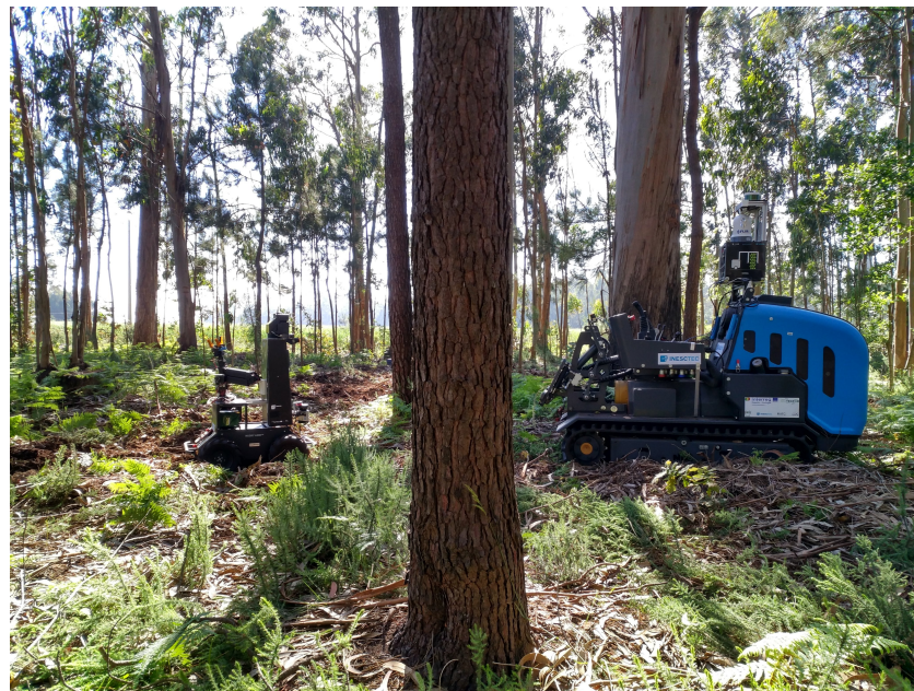
Figure 1. Robotic platforms used to acquire the forest images: on the left side is shown AgRobV16 and on the right side is shown AgRobV18.
