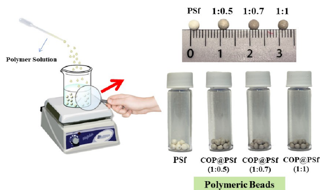
Figure 1. Schematic representation of the procedure for the preparation of polymeric beads.
