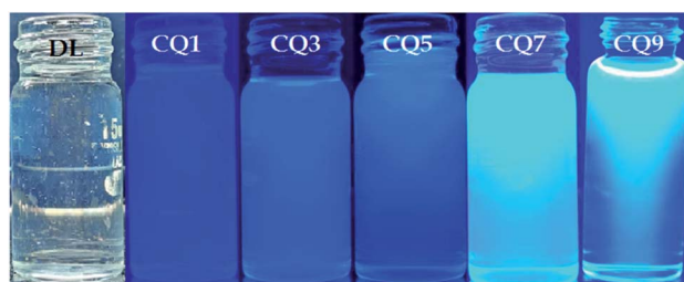
Fig. 2 The images of the prepared C QD under daylight (DL) and long-range UV light (365 nm).
